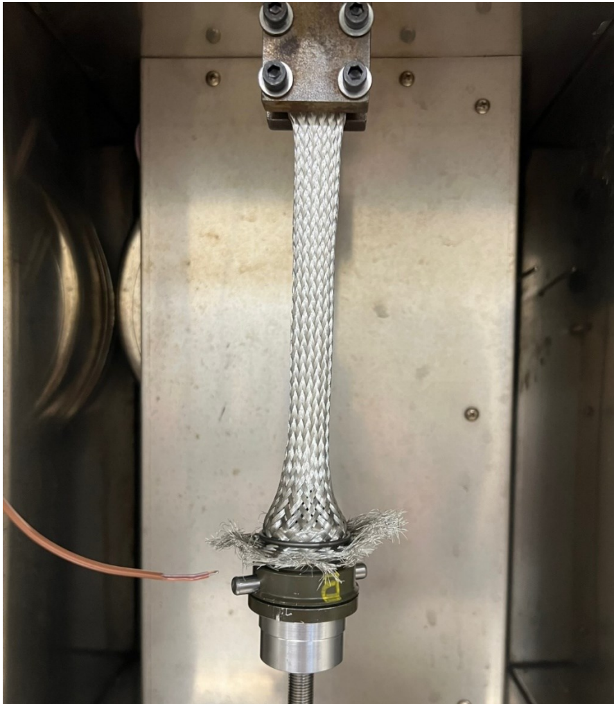
Figure 4 A 16 entry size sample prior to tensile at 23C
