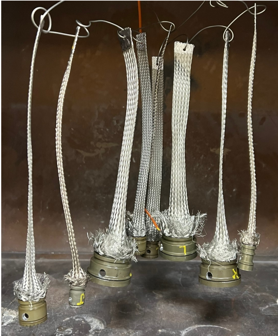
Figure 7 The samples suspended during thermal shock testing in the convection oven
