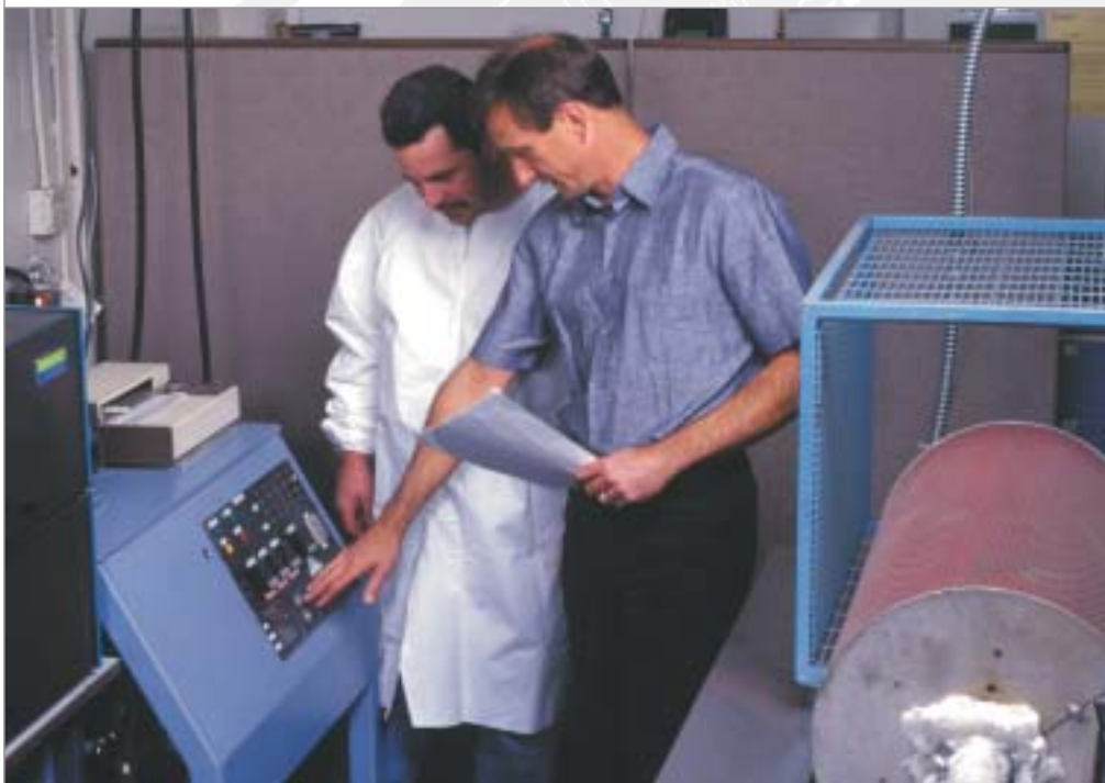
Intrinsic Devices' Tom Borden (right) and Mike DeLuca (left) utilize custom heat treatment equipment to control Nitinol properties.
